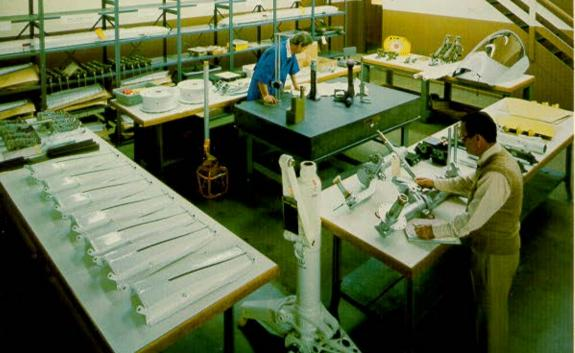
SHEET METAL DEPART-MENT: Equipped for repair, overhaul and production of control surfaces, fuel tanks, canopies, doors, fairings, seats and light metal structures. Equipment: power shears,
